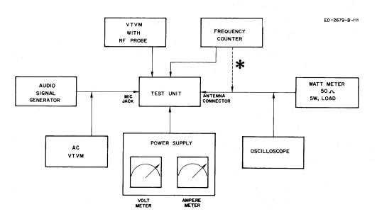
Figure 3-1. Equipment Set-up, Transmitter Alignment
