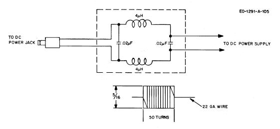
Figure 3-1. Power Line Filter Construction
