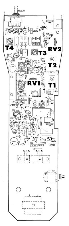
Figure 3-6. Components Adjusted for Receiver Alignment
