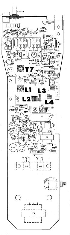
Figure 3-5. Components Adjusted for Transmitter Alignment
