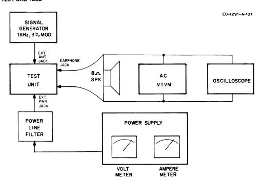
Figure 3-4. Equipment Set-up, Receiver Alignment
