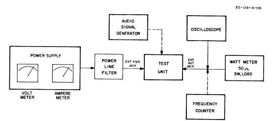
Figure 3-2. Equipment Set-up, Transmitter Alignment
