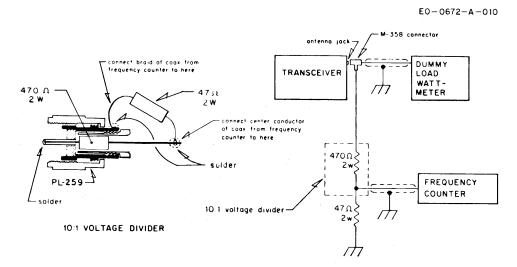
Figure 3-3. Connection of Frequency Counter and Dummy Load
