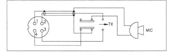
If the microphone to be used is provided with pre-cut leads, they must be revised as follows :
