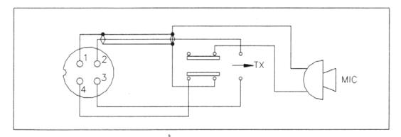
Microphone Schematic Diagram
