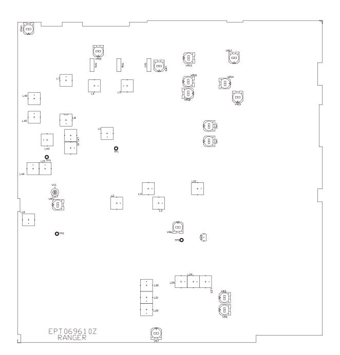
Figure 4-3 Main PCB Adjustment Location
