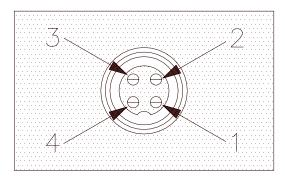
Figure 2-5 Microphone plug pin numbers viewed from rear of pin receptacle.
