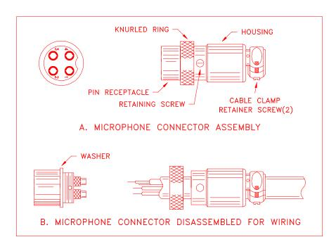
Figure 2-4 Microphone Plug Wiring
