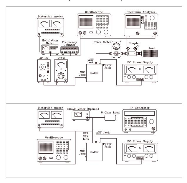
Figure 4-2 Receiver test setup
