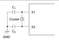
Crystal: 32.768 kHz: MX38T (Nippon Denpa Kogyo)  $C_1:=20~pF\pm20\%$   $C_2:=20~pF\pm20\%$   $R_s:=14~k\Omega$
