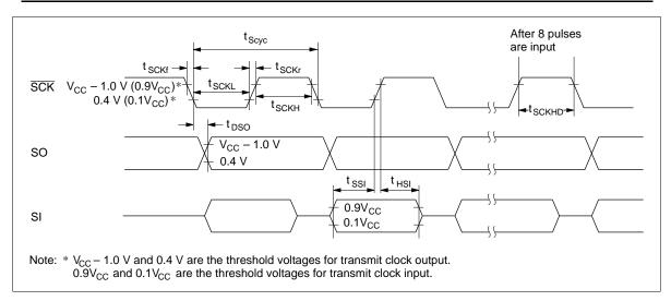
Figure 51 Timing of Serial Interface
