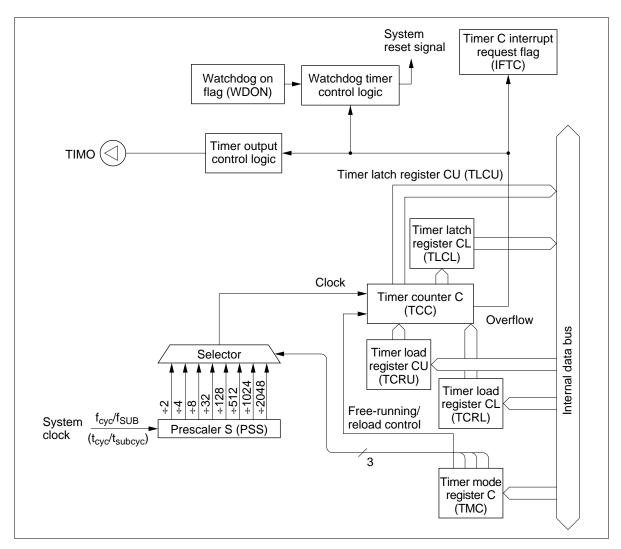
Figure 27 Timer C Block Diagram
