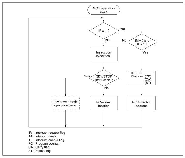
Figure 16 MCU Operating Sequence (MCU operation cycle)
