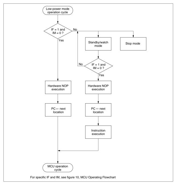
Figure 17 MCU Operating Sequence (low-power mode operation)
