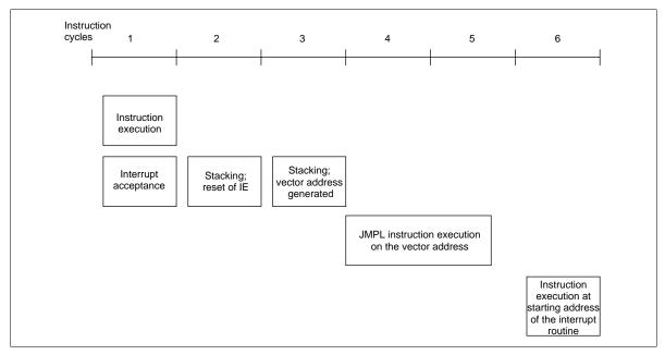
Figure 7 Interrupt Processing Sequence
