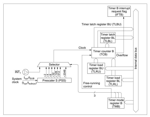
Figure 26 Timer B Block Diagram
