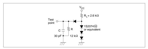
Figure 47 Timing Load Circuit
