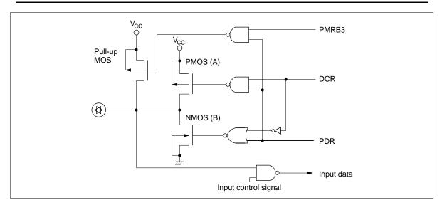
Figure 24 Configuration of the Input/Output Buffer
