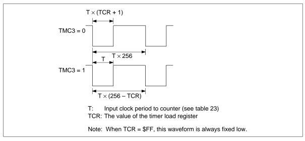
Figure 28 Variable Duty-Cycle Pulse Output Waveform
