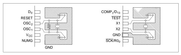
Figure 21 Layout of Crystal and Ceramic Oscillators
