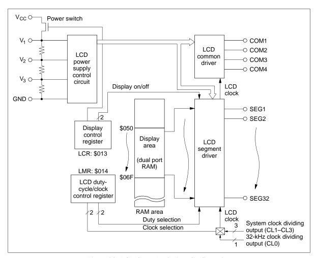
Figure 34 LCD Controller/Driver Configuration
