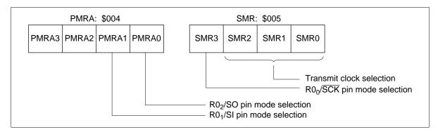
Figure 32 Configurations and Functions of the Mode Registers
