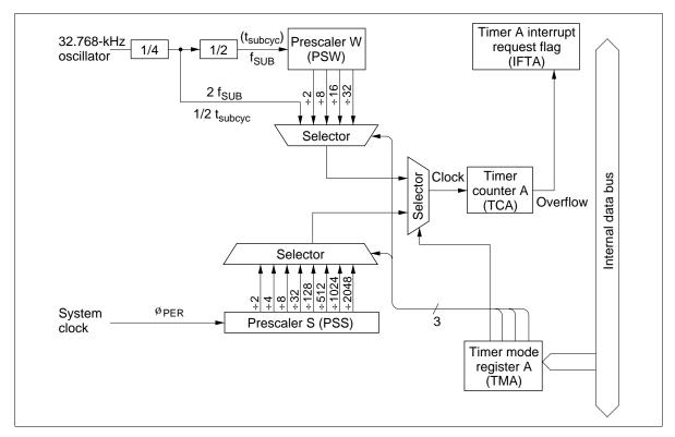
Figure 25 Timer A Block Diagram
