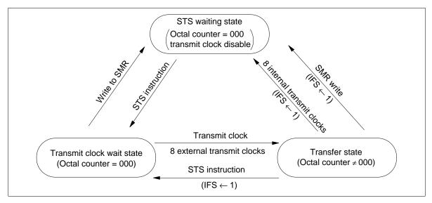
Figure 30 Serial Interface Operation States
