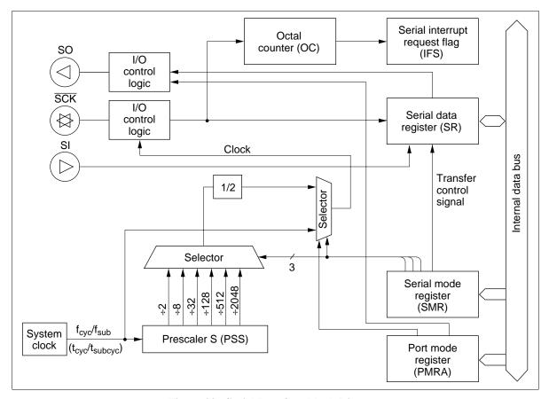
Figure 29 Serial Interface Block Diagram
