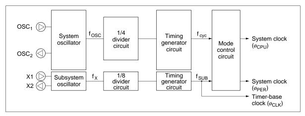
Figure 20 Internal Oscillator Circuit
