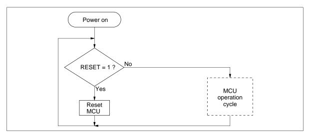
Figure 15 MCU Operating Sequence (power on)
