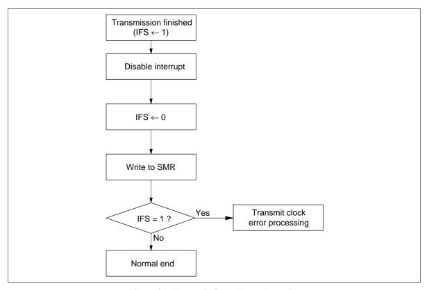
Figure 31 Transmit Clock Error Detection
