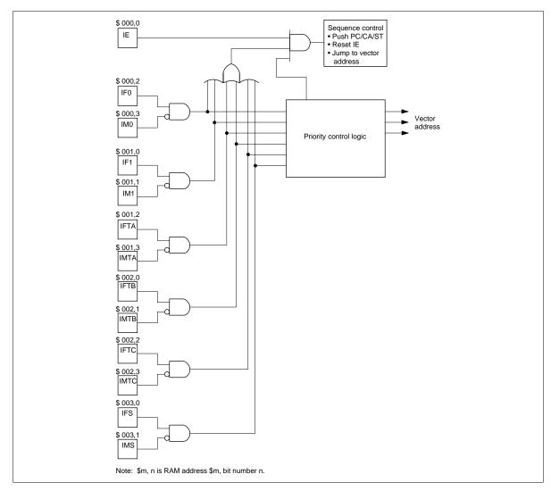
Figure 6 Interrupt Control Circuit Block Diagram
