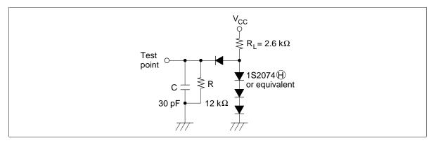
Figure 52 Timing Load Circuit
