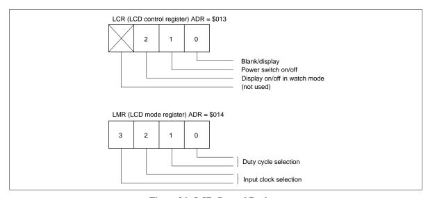
Figure 36 LCD Control Register
