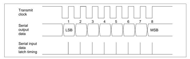
Figure 33 Serial Interface I/O Timing
