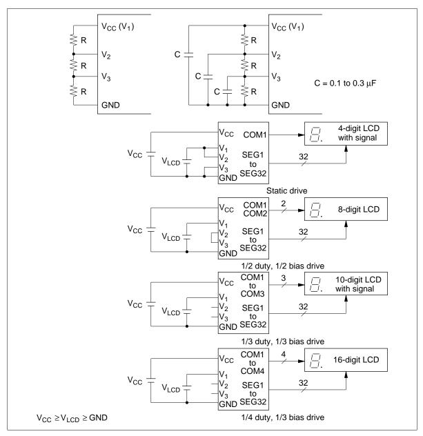
Figure 37 Examples of LCD Connections
