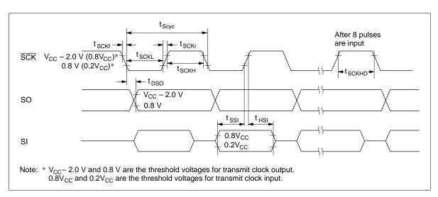
Figure 46 Serial Interface Timing
