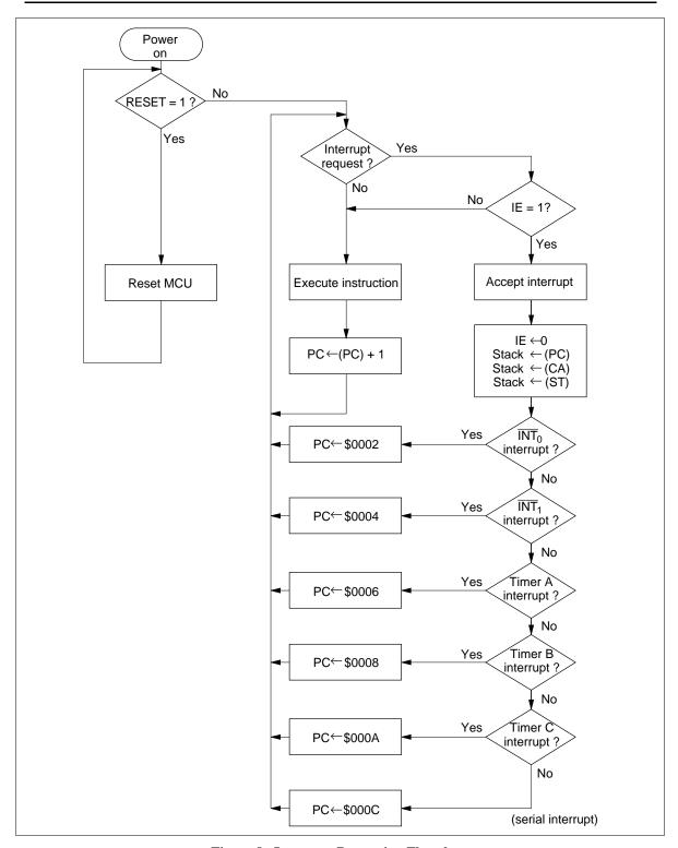
Figure 8 Interrupt Processing Flowchart
