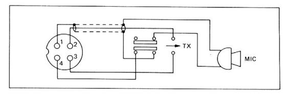
Fig. 3. 侍 samurai microphone schematic.
