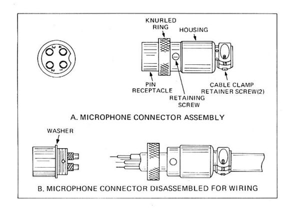
Fig. 4. Microphone plug wiring.
