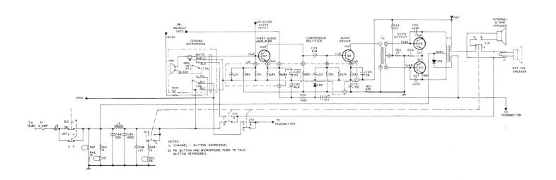
PUBLIC ADDRESS (PA) FUNCTION (SIMPLIFIED SCHEMATIC DIAGRAM)
