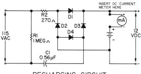
RECHARGING CIRCUIT SCHEMATIC DIAGRAM FIGURE 3-I
