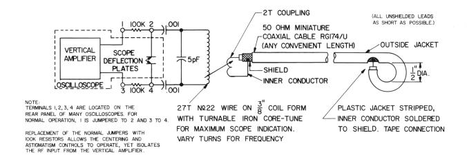
OSCILLOSCOPE RF PICK-UP LOOP AND METHOD OF CONNECTION FIGURE 4-3
