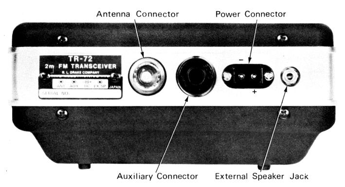
Figure 2-2. Rear Chassis Connectors
