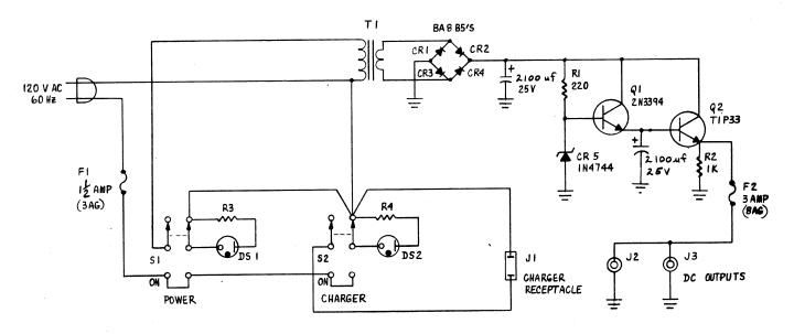
Figure 5-14. Model AC-10 Power Supply Schematic Diagram
