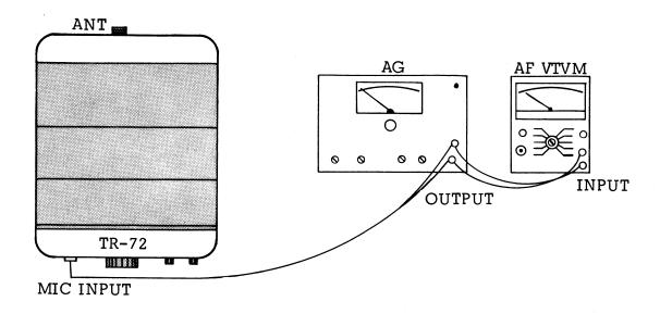
Figure 5-5. Connections for Modulation Adjustment
