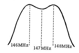
Figure 5-4. Helical Tuner Response Pattern
