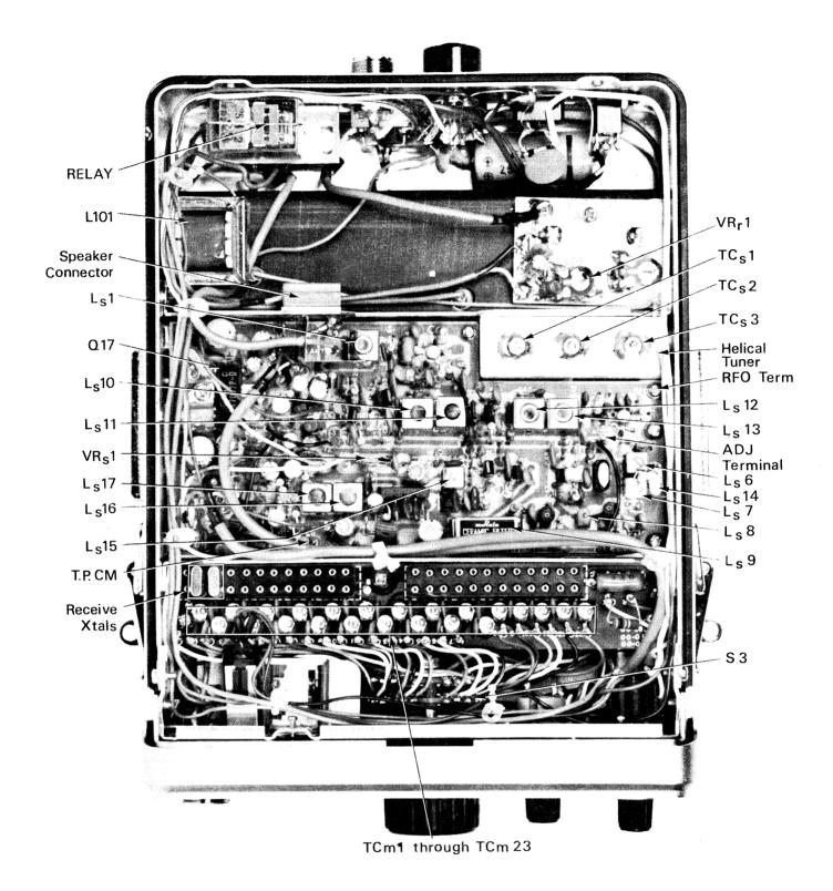
Figure 5—2. Receiver Alignment Locations (Bottom)
