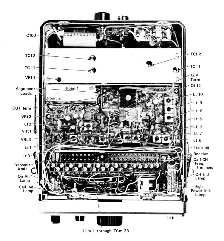
Figure 5–1. Transmitter Alignment Locations (Top)
