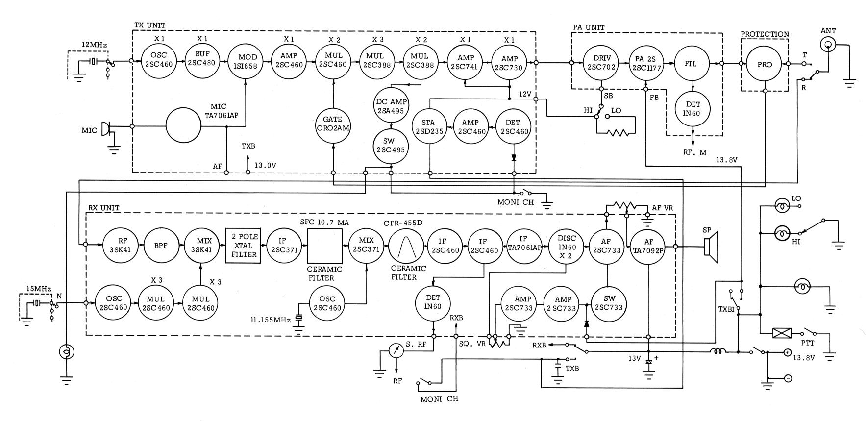
Figure 4-1. TR-72 Block Diagram
