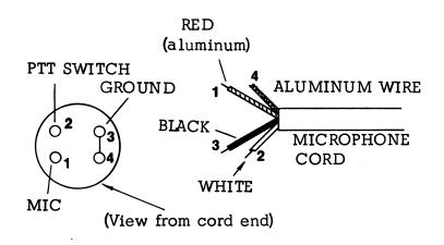
Figure 5-7. Microphone Cord Connections
