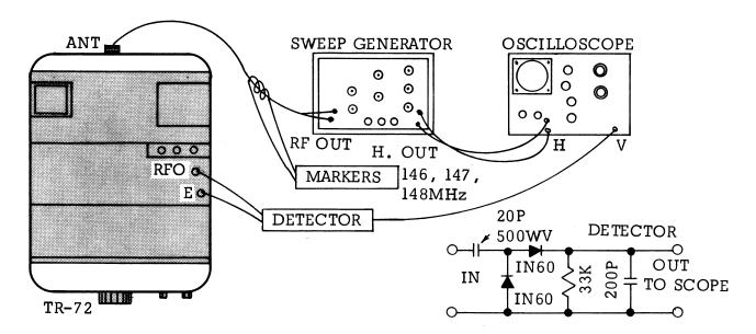
Figure 5-3. Connections for Helical Tuner Alignment
