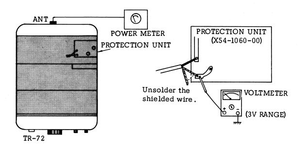
Figure 5-6. Connections for Protection Circuit Adjustment
