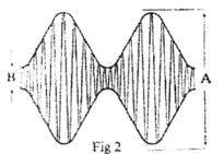
Modulation ratio =  $\frac{A-B}{A+B} \times 100$  [%]
