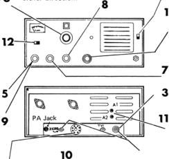
Disconnect the antenna. Zero the meter, with the unit in receive position, by adjusting the control on rear of cabinet.
