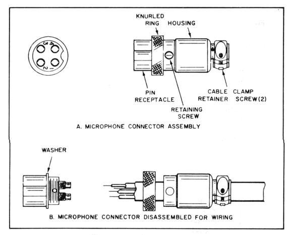
Fig. 2. Microphone plug wiring.
