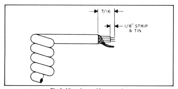
Fig. 1. Microphone cable preparation.
