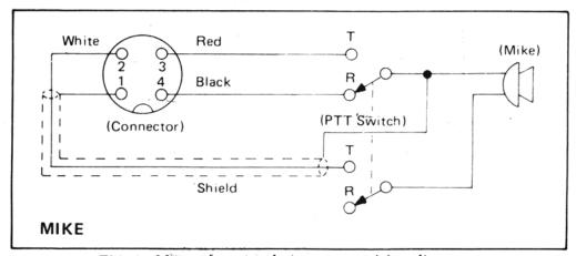
Fig. 4. Microphone and connector wiring diagram.
