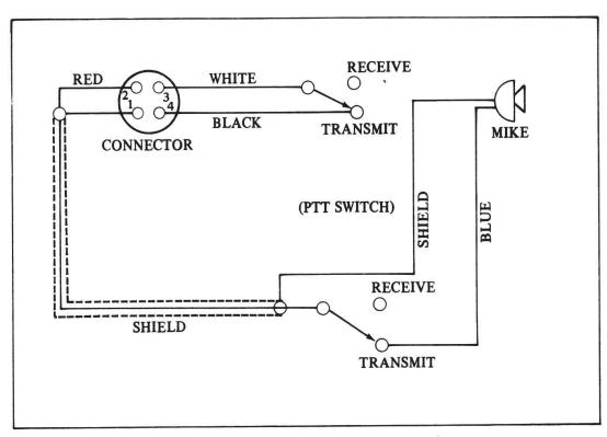
Fig. 3. Microphone and connector wiring diagram.
