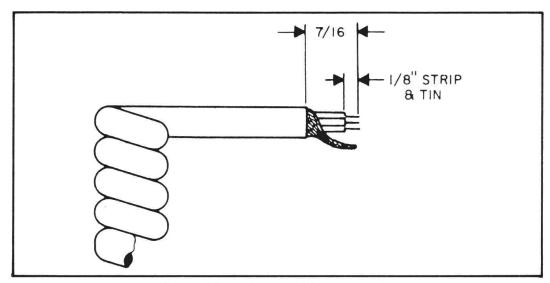
Fig. 1. Microphone cable preparation.
