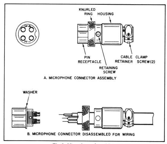
Fig. 2. Microphone plug wiring.
