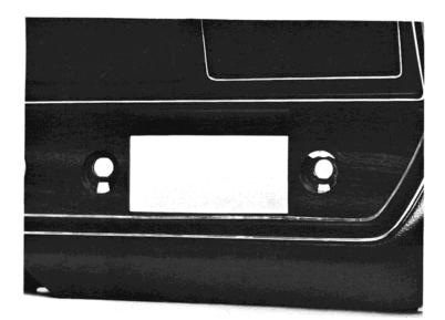
Typical dash opening for rear-removal radio.
