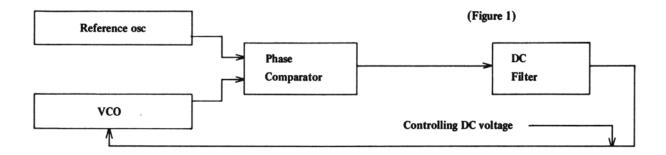
With the above circuit the VCO (Voltage Controlled Oscillator) Frequency is effectively locked to the reference oscillator, and its accuracy is as good as the reference oscillator. Since the CB radio's adjacent channel spacing is 10KHz (or multiple of 5KHz), our purpose should be to preoduce multiple of programable frequencies that are spaced apart by 10KHz.
