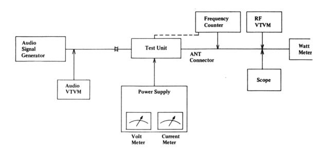
Transmitter Alignment Set Up
