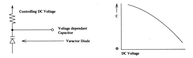
The varactor diode is responsible for setting VCO frequency, and once set it regulates the VCO frequency against the reference.
