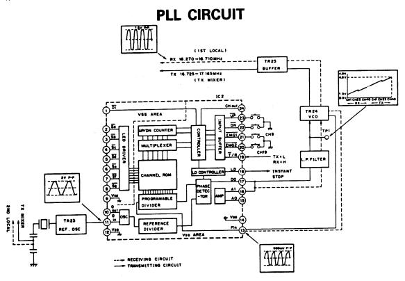
The VCO is an oscillator which controls oscillation frequency in accordance with input voltage change. The VCO output is mixed with a signal in the transmitter or receiver circuitry. A portion of the VCO frequency is fed to IC2 (1/N divider).
