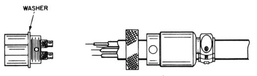
B. MICROPHONE CONNECTOR DISASSEMBLED FOR WIRING
