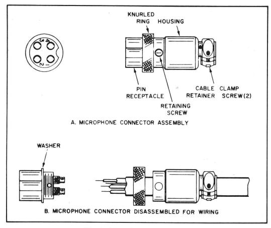
Fig. 2. Microphone plug wiring.
