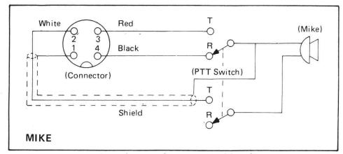
Fig. 3. Microphone and connector wiring diagram.
