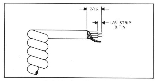
Fig. 1. Microphone cable preparation.
