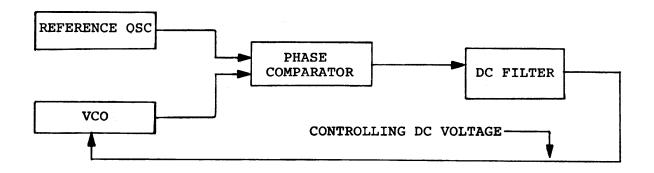
With the above circuit the VCO (Voltage Controlled Oscillator) frequency is effectively locked to the reference oscillator, and its accuracy is as good as the reference oscillator.
