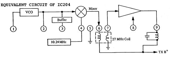
The resulting transmit frequency from pin 9 of IC204 is filtered by L301 and L302. Q301 is an amplifier/switch circuit. When VCO frequency is out of "LOCK" condition pin 14 of IC202 pulls down bias voltage of Q301 to ground disabling Q301 from passing possible illegal frequencies. Q302 is a RF power driver circuit and Q303 is the final RF power amplifier.
