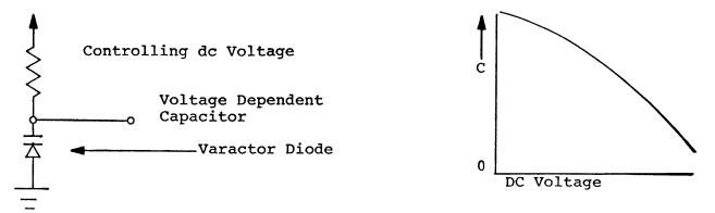
The varactor diode is responsible for setting VCO frequency, and once set it regulates the VCO frequency against the reference. The VCO frequencies are chosen in 16 to 17 MHz range as shown on table 1. To obtain transmit signal the VCO is mixed with 10.24MHz. As an example for channel 1: 10.24 + 16.725 = 26.965MHz
