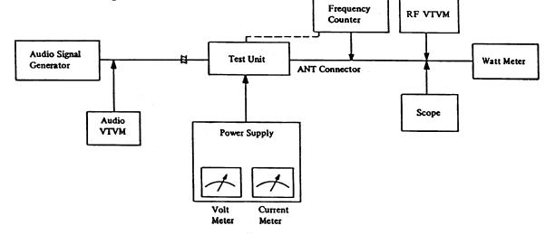
Transmitter Alignment Set Up
