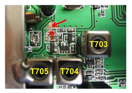
Scrape to expose the circuit traces as indicated above. The large copper area is ground.
