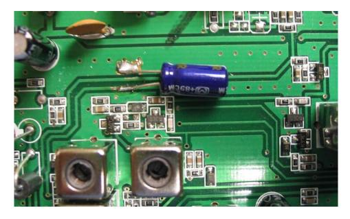
Solder the capacitor as shown. Be sure to observe polarity. Put some glue under the capacitor so that it cannot move.
