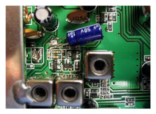
Solder the capacitor as shown. Be sure to observe polarity. Put some glue under the capacitor so that it cannot move.
