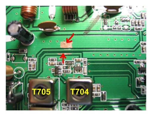
Scrape to expose the circuit traces as indicated above. The large copper area is ground.
