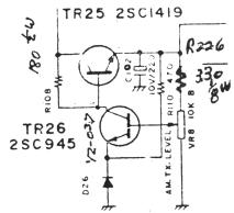
4. ADJUST VR8 FOR 4 WATTS OUTPUT ON A.M. TRANSMIT
