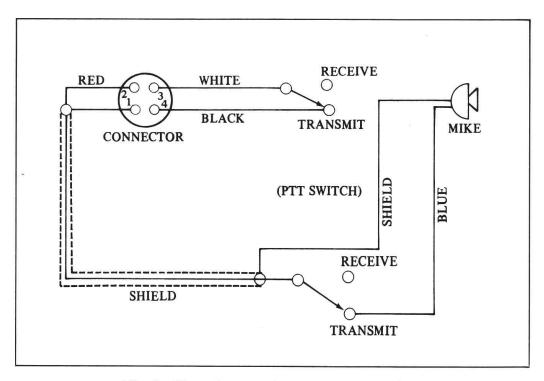
Fig. 3. Microphone and connector wiring diagram.
