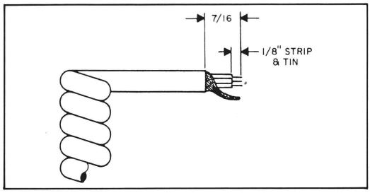
Fig. 1. Microphone cable preparation.
