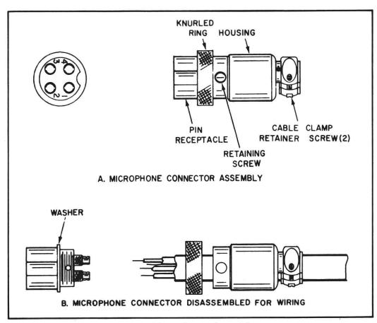
Fig. 2. Microphone plug wiring.
