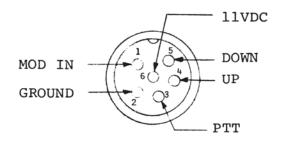
NOTE: FOR TUNING 11VDC IS CONNECTED TO UP OR DOWN BY SWITCH CONTACTS
