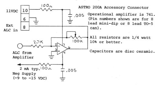
Suggested methods of obtaining the required negative voltage.
