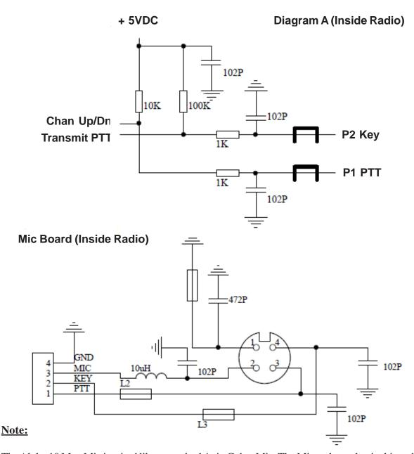
The Alpha 10 Max Mic is wired like a standard 4 pin Cobra Mic. The Microphone that is shipped with the radio has Channel Up/Down Buttons on the front. Initially, there were warnings about the +5VDC on Pin 4 causing damage when using non factory microphones. This is **Not** the case!
