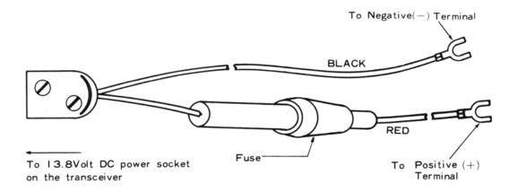
FIGURE 4. CONNECTING DC POWER CORD
