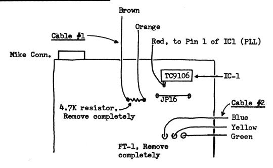
+5KHz Jump Mod - Switch hook-up, or rewire if needed as shown with different type.
