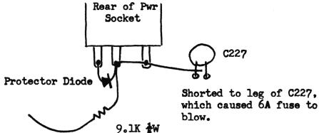
? Used this resistor as piece of jumper, but forgot to cut off the excess leads on both ends, double-check!
