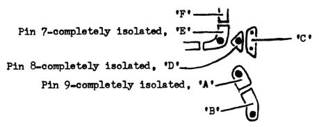
Wire up relay as shown below to switches and PLL etchs (Pts. A - F).
