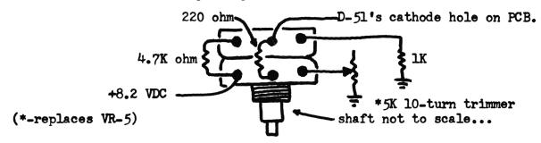
To align the frequency, center up the knobs and adjust all three modes for center slot. Now, decide how much slide you will need. The slide is adjustable from 5KHz to 20KHz, but only in the down portion. Upwards amount of slide will remain the same. Reason: Voltage is remaing constant at the top of control; but can adjust resistance to ground with the 10-turn trimmer; thus can control the amount of voltage drop. In most cases the slide up will be about 7KHz and down about 13KHz.
