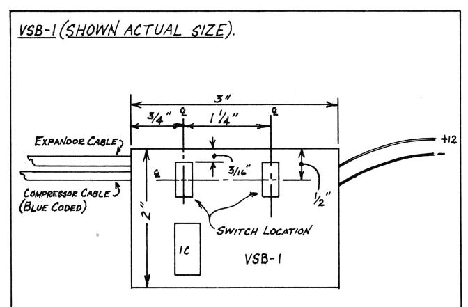
DRILL TWO(2) 14" DIA. HOLES 14" APART FOR SWITCHES IN A CONVENIENT PLACE TO MOUNT VSB-1. MAKE SURE THERE IS ENOUGH CLEARANCE SO BOARD WON'T TOUCH ANYTHING ELSE IN RADIO.
