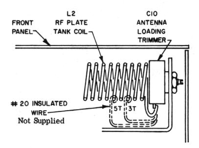
FIG. 2 TOP VIEW OF TANK COIL
