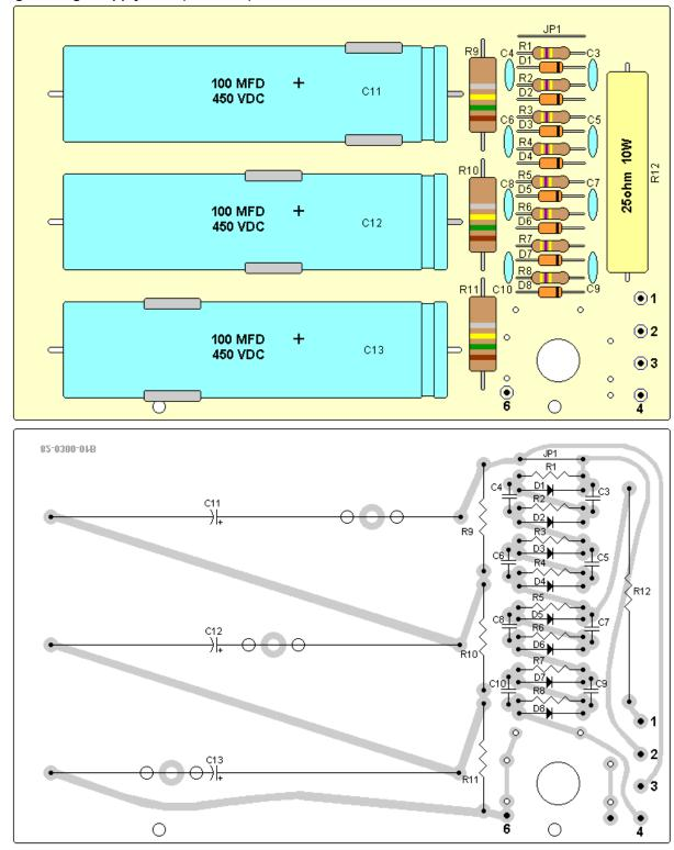
PRIDE DX300 Bi Linear Amplifier HIGH Voltage Power Supply PCB (Board #2) 82-0300-01B
