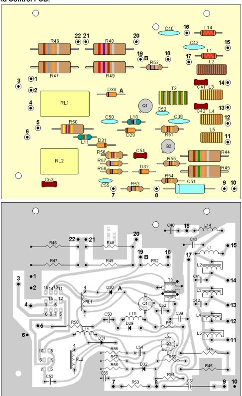
PRIDE DX300 Bi Linear Amplifier RF Relay and Control PCB 82-0300-03 Copyright © 2004, CBTricks.com All Rights Reserved Rev.# 1.2
