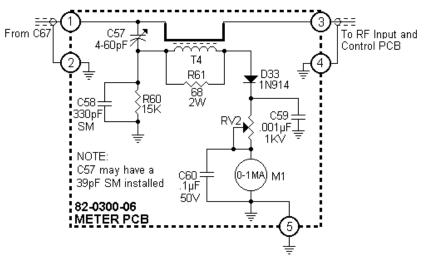
Figure 3-6 Wattmeter Circuit
