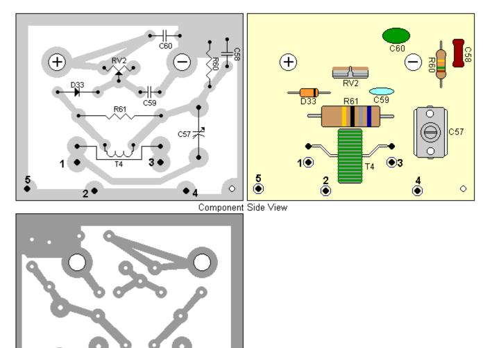
PRIDE DX300 Bi Linear Amplifier Meter PCB 82-0300-02B
