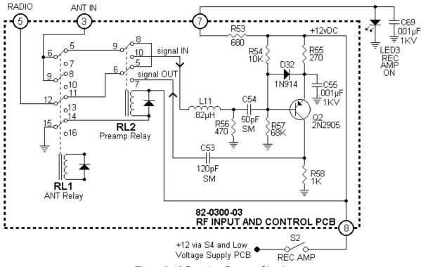
Figure 3-42 Receiver Preamp Circuit
