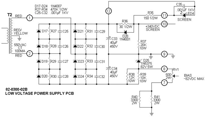
Figure 3-2 Screen and Bias Voltage Power Supply
