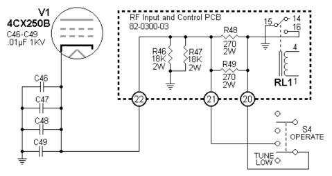
Figure 3-41 Cathode Circuit
