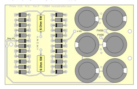
The Kit includes all the parts to build a single PCB HV Power Supply that replaces both HV PCB in a Pride DX300. This PCB lets you completely remove the original two H.V. circuit boards and install the single-piece replacement.
