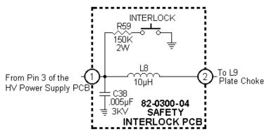
Figure 3-5 Safety Interlock Circuit
