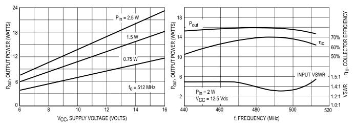
Figure 4. Power Output versus Supply Voltage
