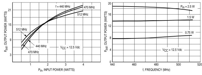
Figure 2. Output Power versus Input Power
