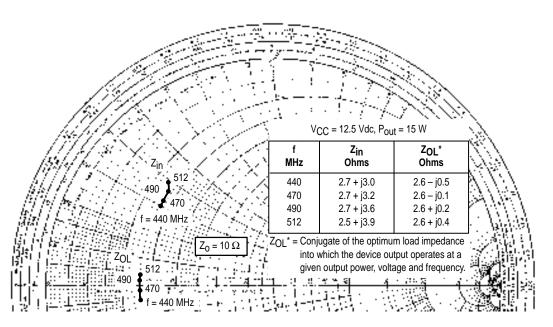
Figure 6. Series Equivalent Input and Output Impedance
