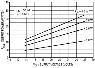
Figure 4. Output Power versus Supply Voltage
