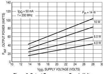
Figure 6. Output Power versus Supply Voltage
