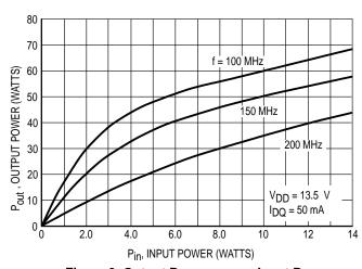
Figure 3. Output Power versus Input Power
