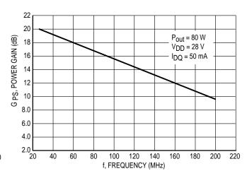
Figure 7. Power Gain versus Frequency
