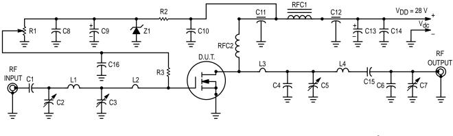
C1, C15 — 470 pF Unelco C2, C3, C5 — 9–180 pF, Arco 463 C4, C6 — 15 pF, Unelco C7 — 5–80 pF, Arco 462 C8, C10, C14, C16 — 0.1  $\mu$ F C9, C13 — 50  $\mu$ F, 50 Vdc C11, C12 — 680 pF, Feed Through L1 — #16 AWG, 1–1/4 Turns, 0.3" ID L2 — #16 AWG Hairpin 1" long
