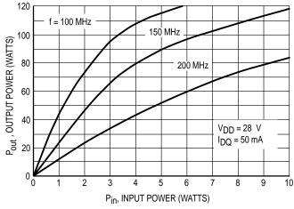
Figure 2. Output Power versus Input Power
