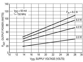
Figure 5. Output Power versus Supply Voltage
