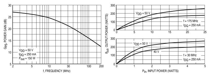
Figure 7. Power Gain versus Frequency
