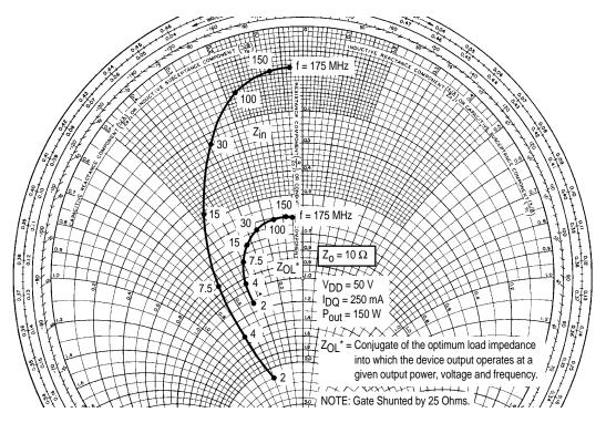
Figure 10. Series Equivalent Impedance
