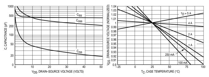
Figure 3. Capacitance versus **Drain-Source Voltage**
