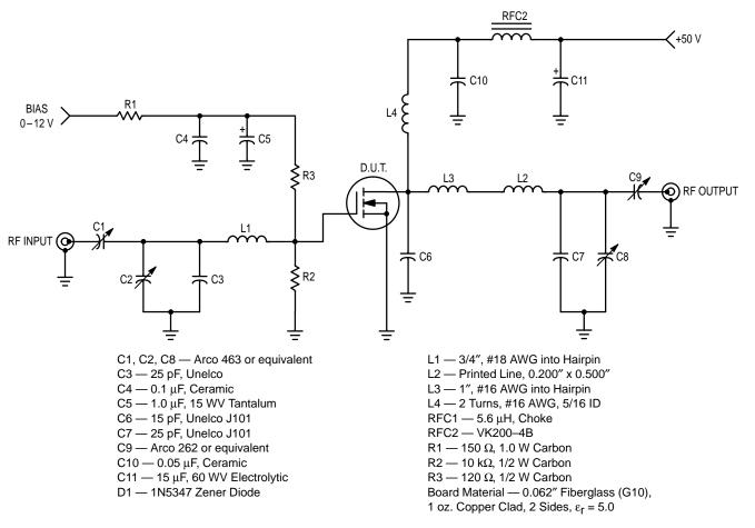
Figure 2. 175 MHz Test Circuit
