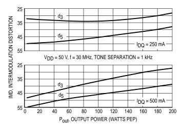
Figure 9. IMD versus Pout
