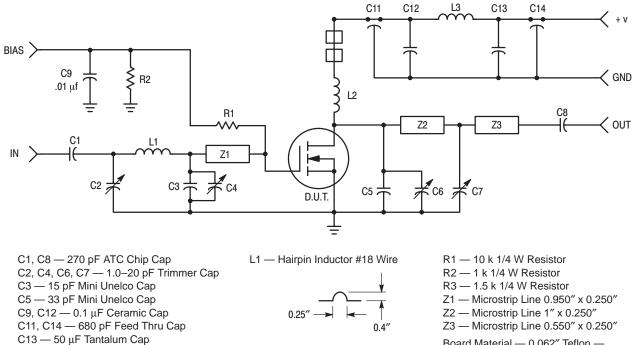
Board Material - 0.062" Teflon fiberglass,  $\varepsilon_r$  = 2.56, 1 oz. copper clad both sides
