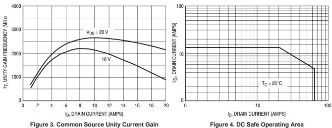
**Frequency versus Drain Current**
